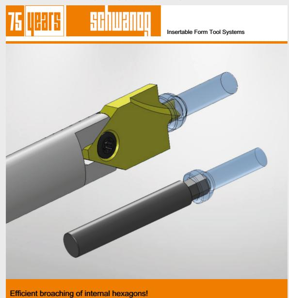
One of the classic applications in the medical industry is the machining of screw heads on implants. Most orthopedic implants have an internal hex.
