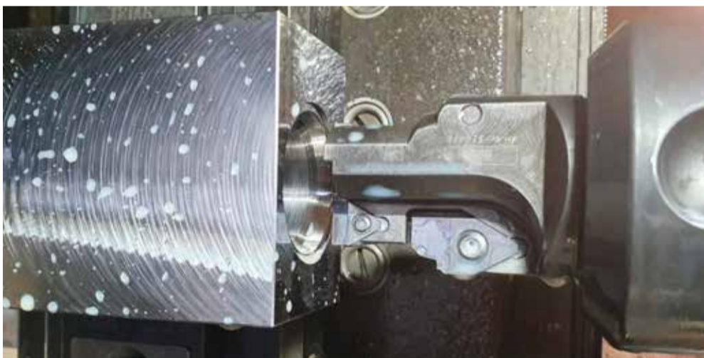
Drilling of valve block using 2 Schwanog PWP insertable form drills
