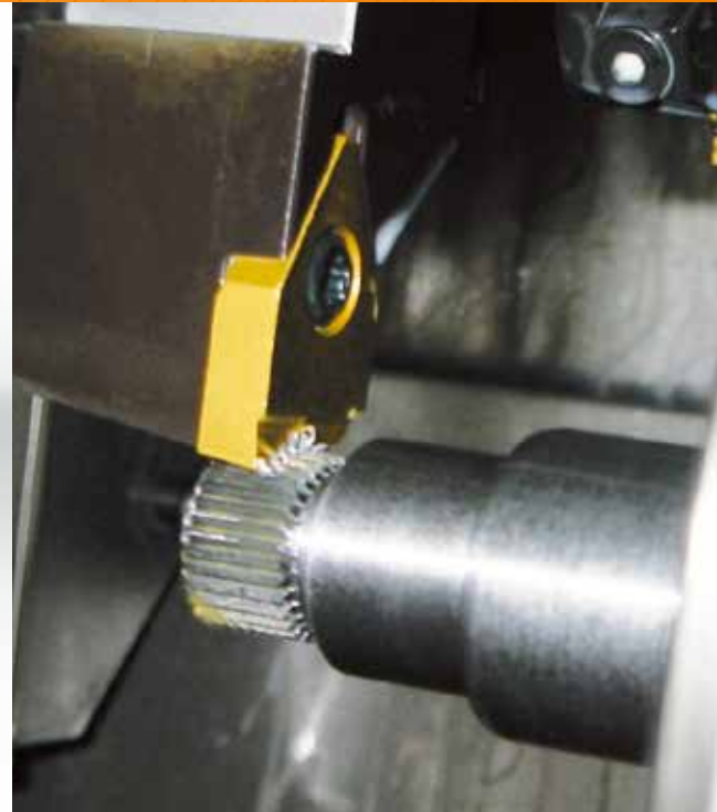
Machining of turned parts with serration.
