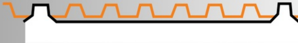
Two finish threader for long threads
