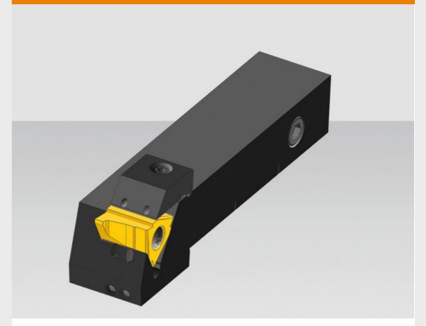
By targeted expansion of the OD grooving application of the 3-cutting edge WEP system, it is now possible to achieve cutting widths of up to 16 mm with a holder height of 20 mm and higher.
