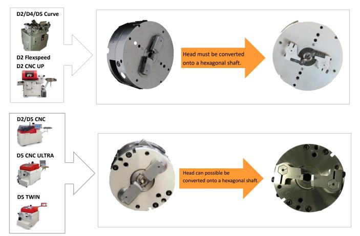
For all other machines the conversion is eliminated. These machines are already equipped with the hexagonal shaft.
