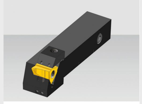
By targeted expansion of the OD grooving application of the 3-cutting edge WEP system, it is now possible to achieve cutting widths of up to 16 mm with a holder height of 20 mm and higher.
