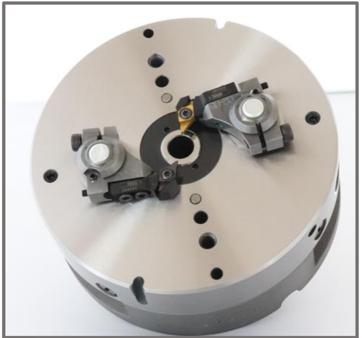
CONVERTED VENTURA HEAD D2 120 WITH HEXAGONAL SHAFT
