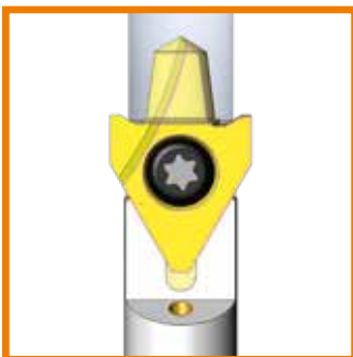
Drilling of taper with PWP insert
