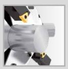
OD Grooving for rotary transfer machines
