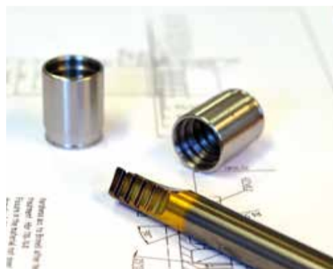
Schwanog solid carbide grooving tool for machining inner contours
