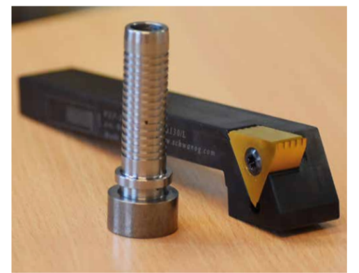
Schwanog WEP system for external plunge cutting of grooves
