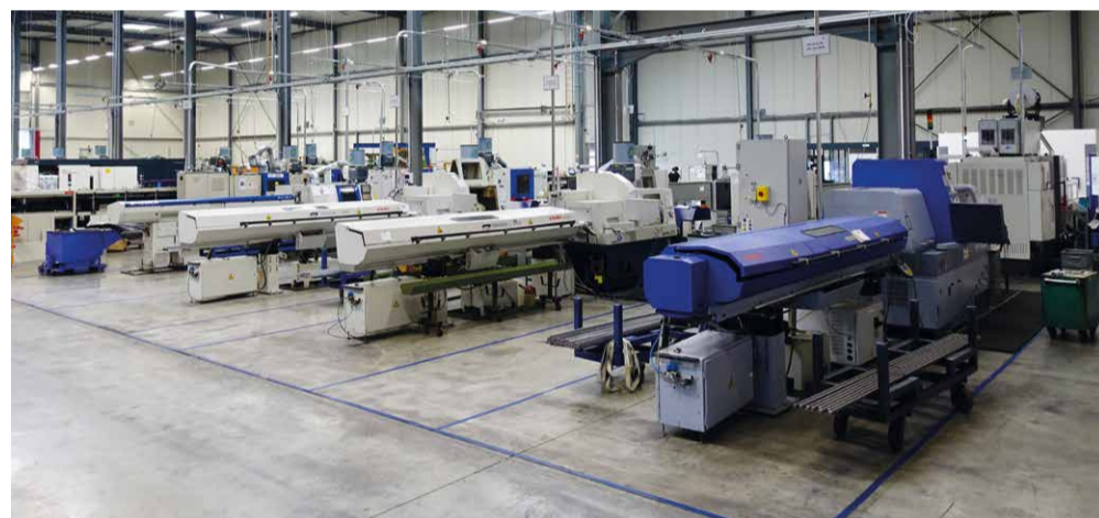
WIGGENTech's machine park consists of around 20 multi-spindle and single-spindle lathes
