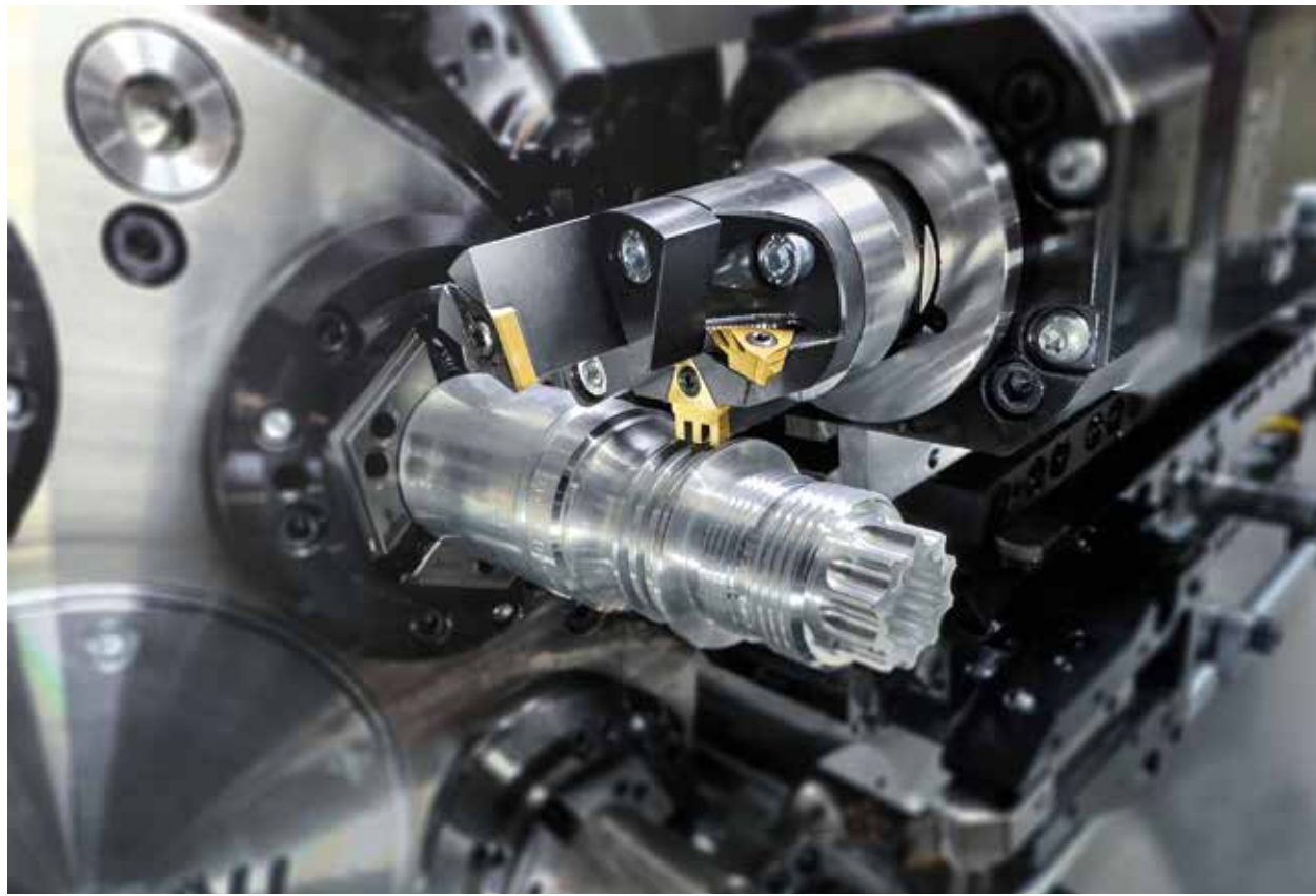
HDT 2.0 combination tool, form-grooving tool in machining position
